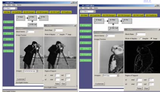
Low-pass filtering of a natural image High-pass filtering of a natural image
